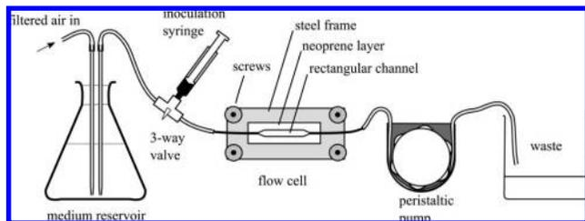
**Figure 1.** Biofilms were cultivated in a flow cell, consisting of a rectangular channel with tapered ends, cut into a Neoprene sheet, and sandwiched between a glass microscope slide and a coverslip in a rubber-padded steel frame. The biofilm was fed with a sterile aerated medium, using a peristaltic pump.
